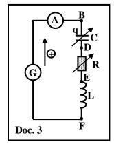
alternating sinusoidal voltage  $u_G = u_{BF} = 3 \sin(\omega t)$ , ( $u_G$  in V, t in s) and  $\omega = 314 \text{ rad/s}$ .
