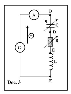
This circuit is connected across a generator (G) maintains across its terminals an alternating sinusoidal voltage  $\mathbf{u}_G = \mathbf{u}_{BF} = 3\sin(\omega t)$ , ( $\mathbf{u}_G$  in  $\mathbf{V}$ , t in s) and  $\omega = 314$  rad/s. The expression of the current in the circuit is  $\mathbf{i} = \mathbf{I}_m \sin(\omega t + \varphi)$ .
